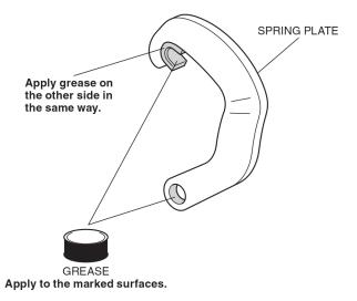
8. Install the springs to the spring plate as shown.
