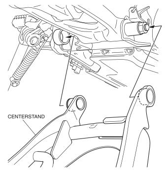
Install the circlip and washer as shown.
