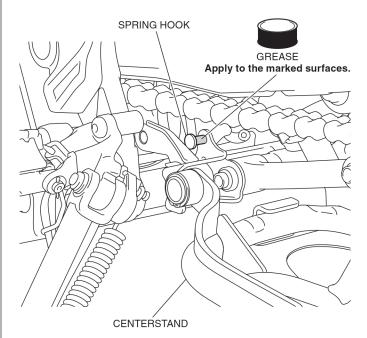
10. Install the spring plate as shown.
