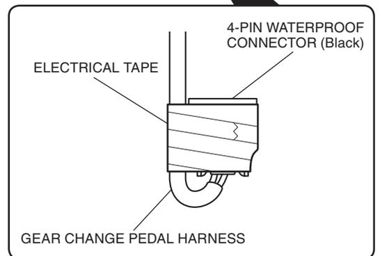
6. Install the gear change pedal as shown.
