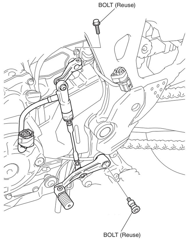
9. Connect the gear change pedal harness as shown.
