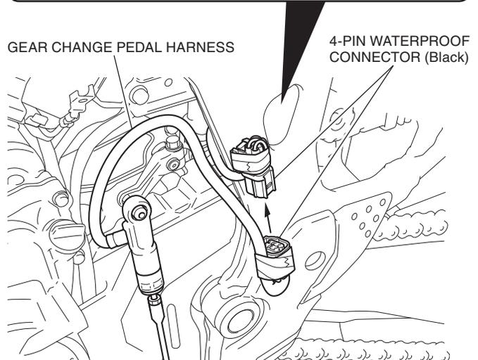
10. Secure the gear change switch harness with the wire ties as shown.
