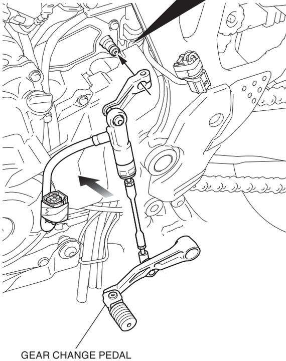
7. Apply grease to the bolt as shown.
