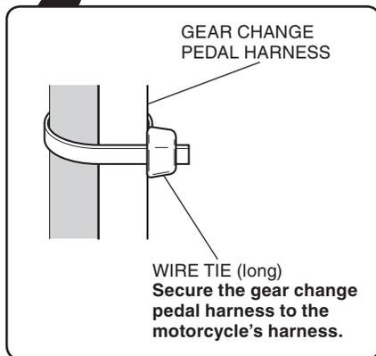
11. Secure the gear change switch harness with the wire tie as shown.
