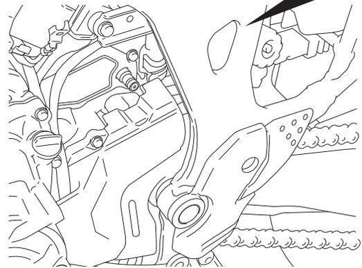
5. Secure the gear change pedal harness in the position of the dimension shown.
