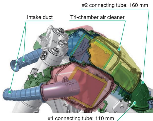
Fig. 28 Configuration of air intake system
