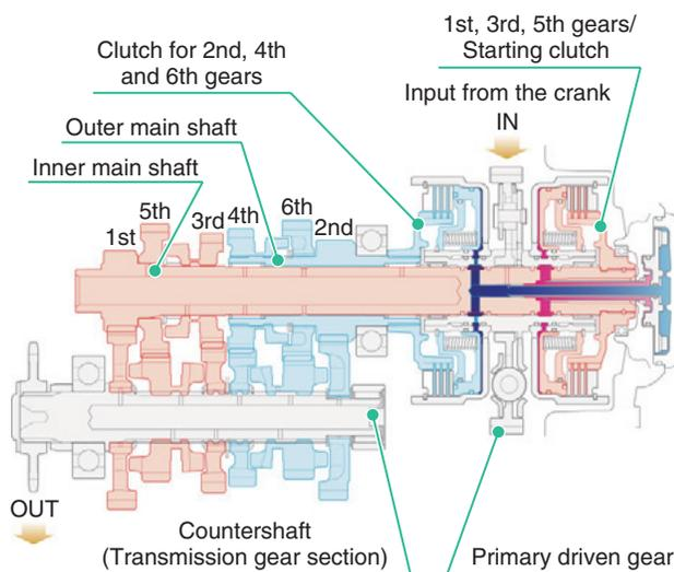
Fig. 20 DCT system
