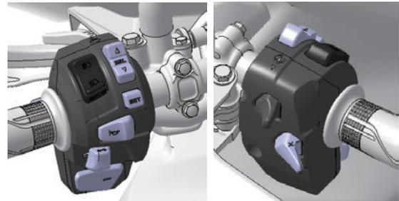
(a) Left handle switch (b) Shift up switch for DCT on the back side of the left handle
