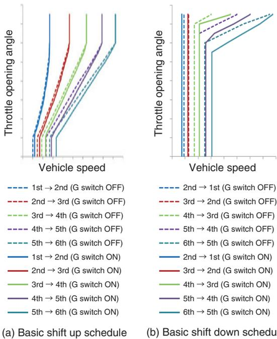
Fig. 23 Shift schedule in AT mode with G-switch on or off
