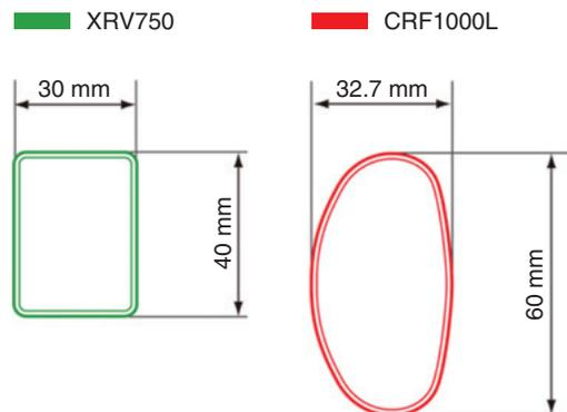
Fig. 8 Comparisons of frame pipe cross section
