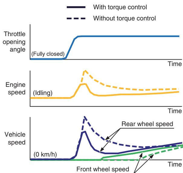
Fig. 27 Honda selectable torque control operation at start
