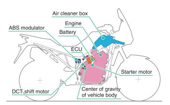
Fig. 2 Layout of key components
