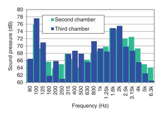
Fig. 30 Measurement results of exhaust sound pressure
