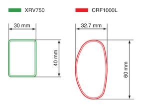
Comparisons of frame pipe cross section Fig. 8
