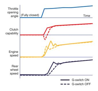
Fig. 22 Clutch capability control with G-switch
