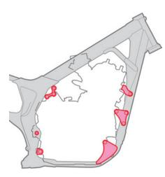
Fig. 9 Six engine hanger locations
