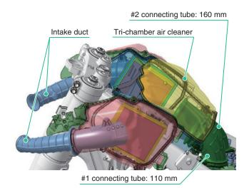
Fig. 28 Configuration of air intake system
