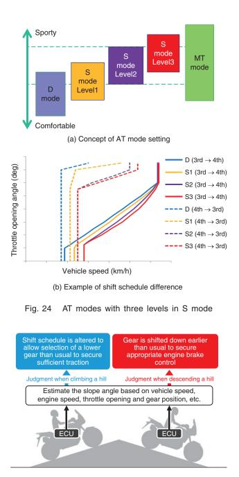
Fig. 25 Image diagram of gear-shifting control at uphill and downhill
