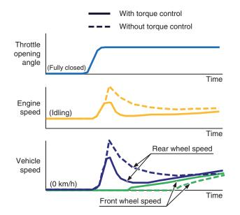
Fig. 27 Honda selectable torque control operation at start
