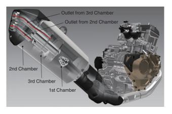
Fig. 29 Structure of muffler
