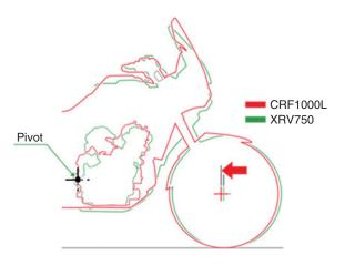
Fig. 4 Comparison of front axle positions
