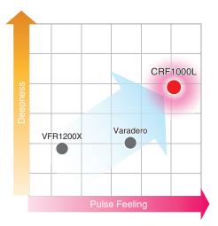
Fig. 31 Evaluation results of exhaust sound
