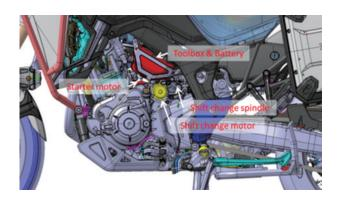
Fig. 21 Location of DCT shift motor
