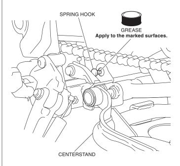
10. Install the spring plate as shown.
