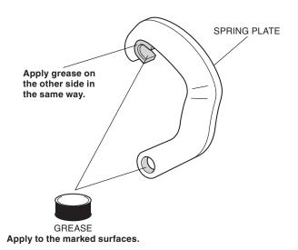
8. Install the springs to the spring plate as shown.
